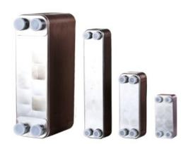
Made of a corrugated plate pack without gaskets, welded together with copper brazing in a vacuum
